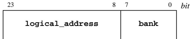
If the pointer is 4 bytes the address layout is:
